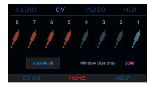
There are 8 non-polar 0-10v CV input jacks on the back panel of the synth, visibly labeled, all of which can be used simultaneously. When a CV cable is plugged into the synth the corresponding icon on the CV I/O page will illuminate.
